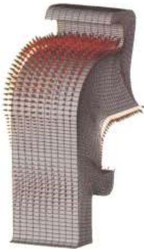
Reaction forces in the uplift restraint of Alternativ I
